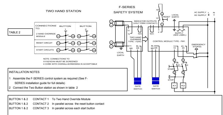
IMPORTANT: Ensure that Button 1 & Button 2 (Contact 2) are connected in parallel across the reset button to ensure the correct operation
