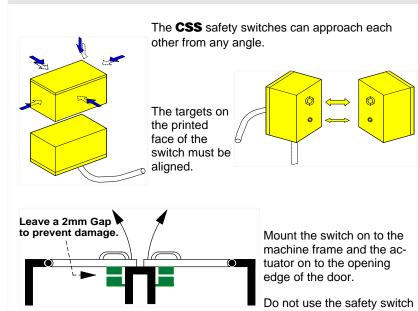
Always try to mount the switch on nonferrous material. Ferrous material will reduce the switching distance.
