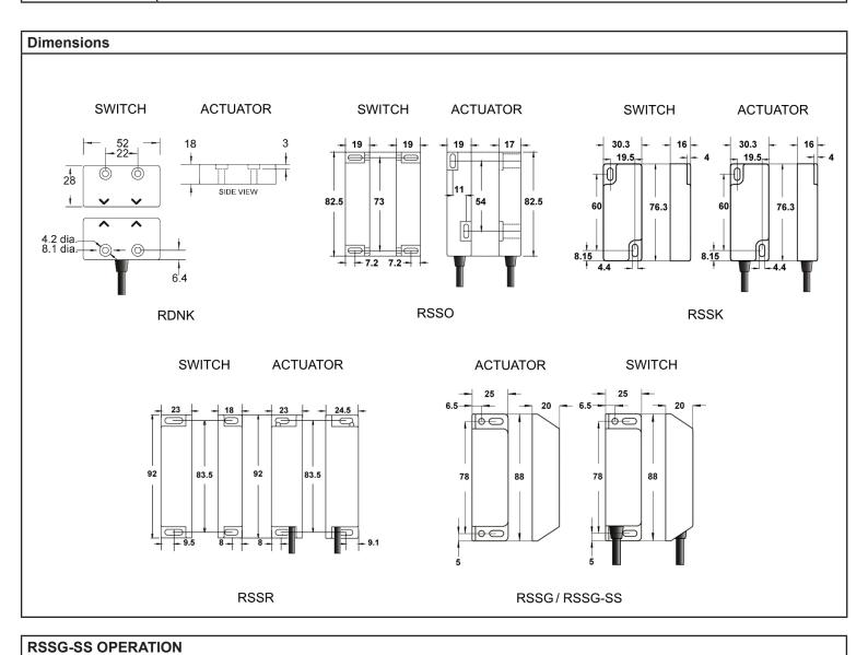
The N/O contacts on the RSS-SERIES switches are open when the actuator is away from the switch.
