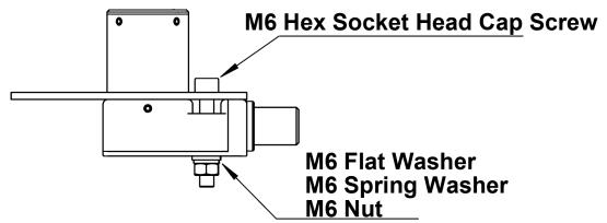
The recommended torque to tighten the fixings is 8 to 10Nm.
