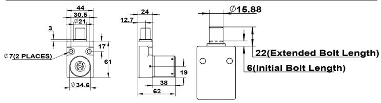
When the key is in the trapped position, the bolt length is 6 mm.
