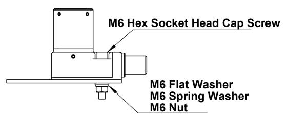
Back of board mounting: 2 x M6 Hex socket head cap screws / minimum screw length = 37mm + panel thickness 2 x M6 Spring washer, 2 x M6 Flat Washer, 2 x M6 Nut.
