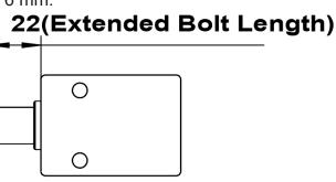
When the key is released from the BL1 Lock, the bolt length is 22 mm.
